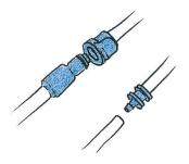
Use connectors to extend the tubes length or to combine different MULTIPADs.
